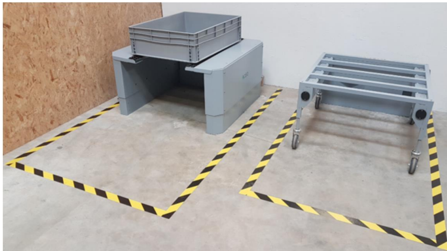
Figure 7: Load transfer areas must be marked as OHZs, e.g. using tape, paint, signs, etc.
