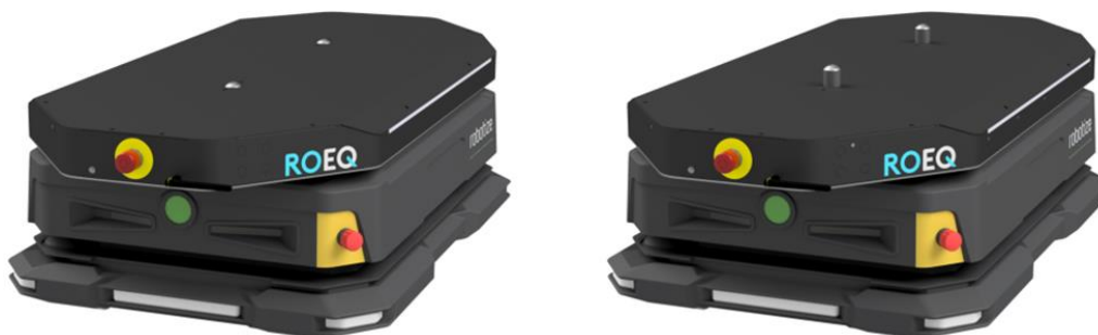
Figure 1: Left: Pins lowered. Right: Pins raised.
